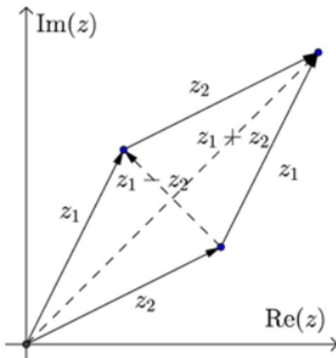
This result has a geometric interpretation. By interpreting complex numbers  $z_1$  and  $z_2$  as vectors, we obtain a parallelogram with diagonals whose vectors are  $z_1 + z_2$  and  $z_1 - z_2$ . This result then shows that the sum of the squares of the lengths of the four sides of a parallelogram equals the sum of the squares of the lengths of the two diagonals.
